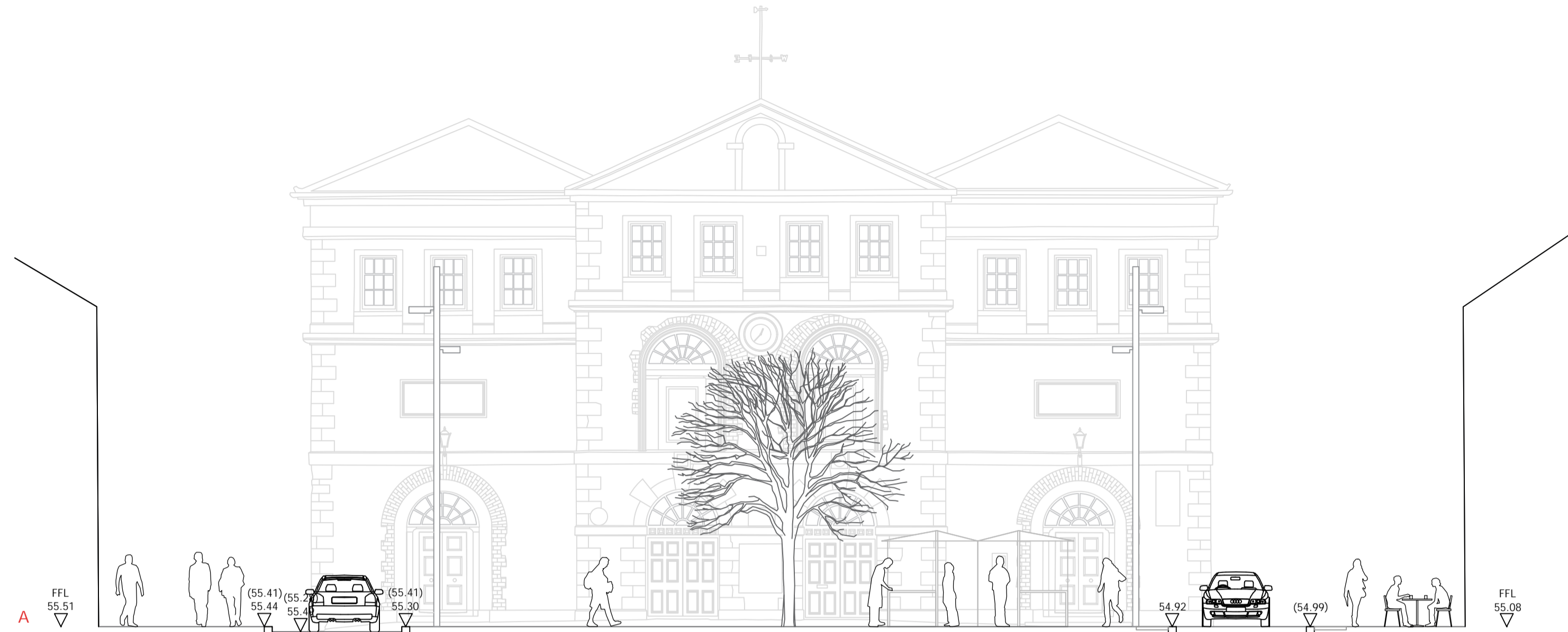
Section/Elevation A-A Showing widened footpaths, one way carriageways and street lighting Scale 1:100
